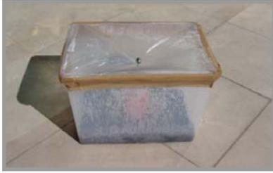
5. Place the solar still in a still and sunny location (it may pay to check with groundsman to find the best position – wind can cause the cling wrap to flap about so that the droplets miss the cup).
