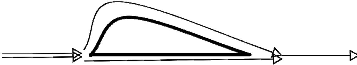
From here there are two important things to know. First, as air moves faster it creates less pressure. Second, things want to move from areas of high pressure to areas of low pressure. All of this simply means the wing is going to want to move upwards and that is how we get and the plane is able to stay in the air!
