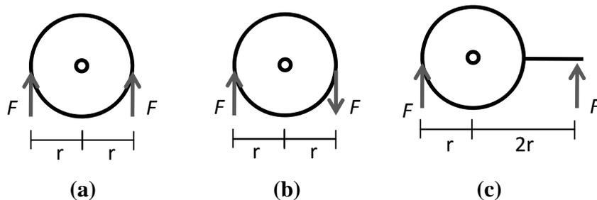
diagram (a) shows forces acting in the same direction and at the same distance from the axis of rotation, but on different sides of the axis of rotation. These forces will not rotate the object because the net torque is zero:
